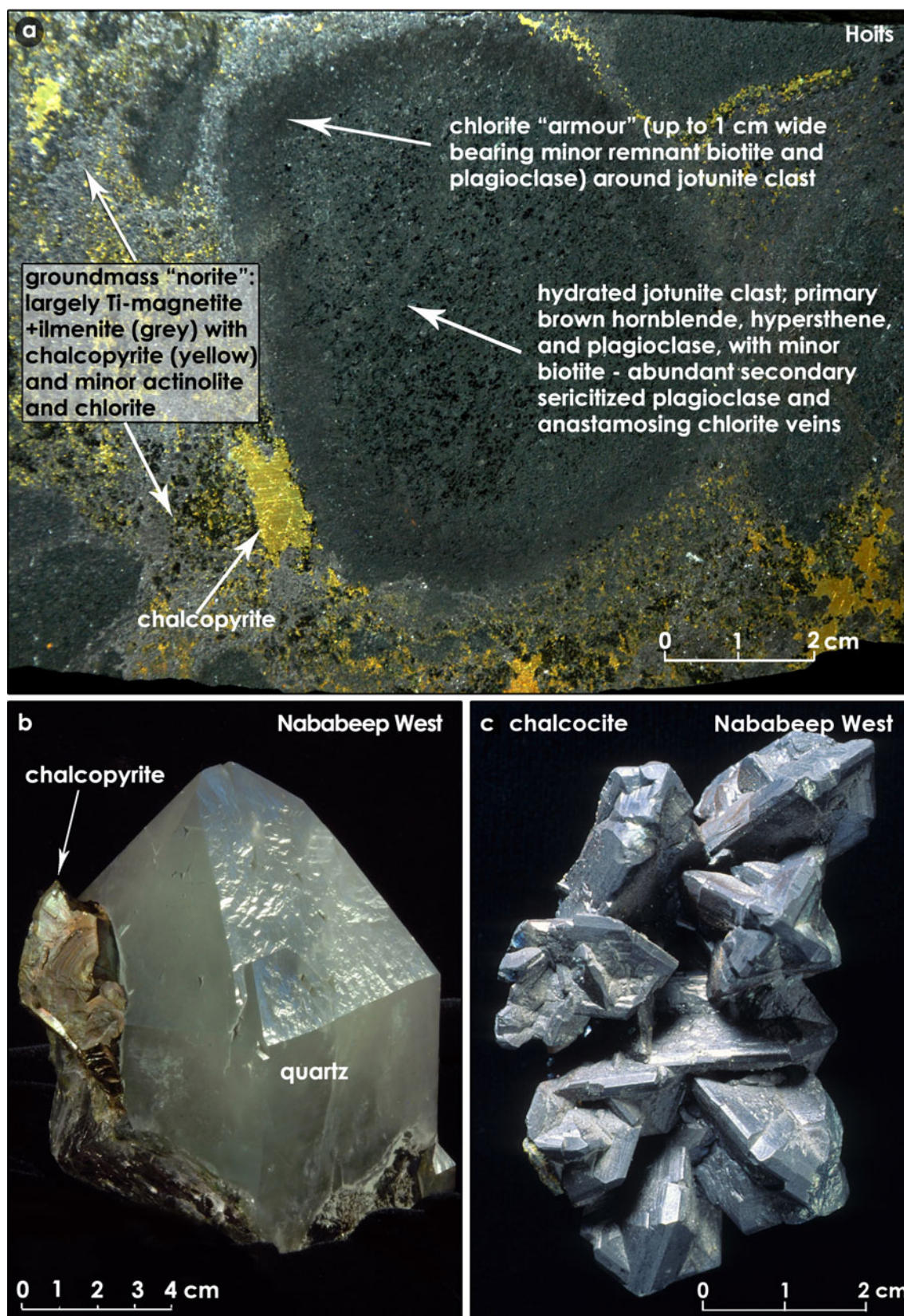
Fig. 16 Koperberg Suite. Hoits-type ore: a cognate xenolith of jotunite (rimmed by chlorite) in norite bearing chalcopyrite, ilmenite, and Ti-magnetite, 295 m level, Hoits Mine; b quartz with chalcopyrite,
