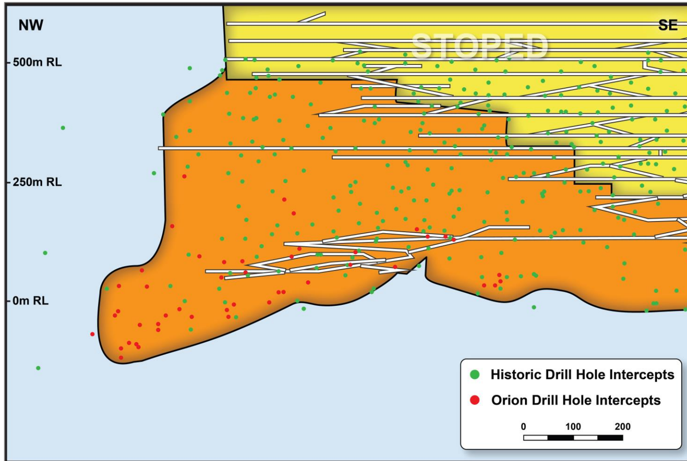
JORC (2012) Table 1: JORC Table 1: Figure 3A: Longitudinal projection of the North-West Resource area of the Prieska deposit, showing the intersection points of the drillholes used to estimate the Mineral Resource.
