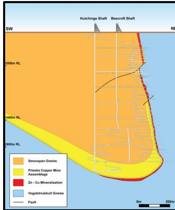
JORC (2012) Table 1; JORC Table 1: Figure 2A: Simplified geological section through the Prieska deposit showing structure and relative location of the Deep Sulphide Target below the old workings.
