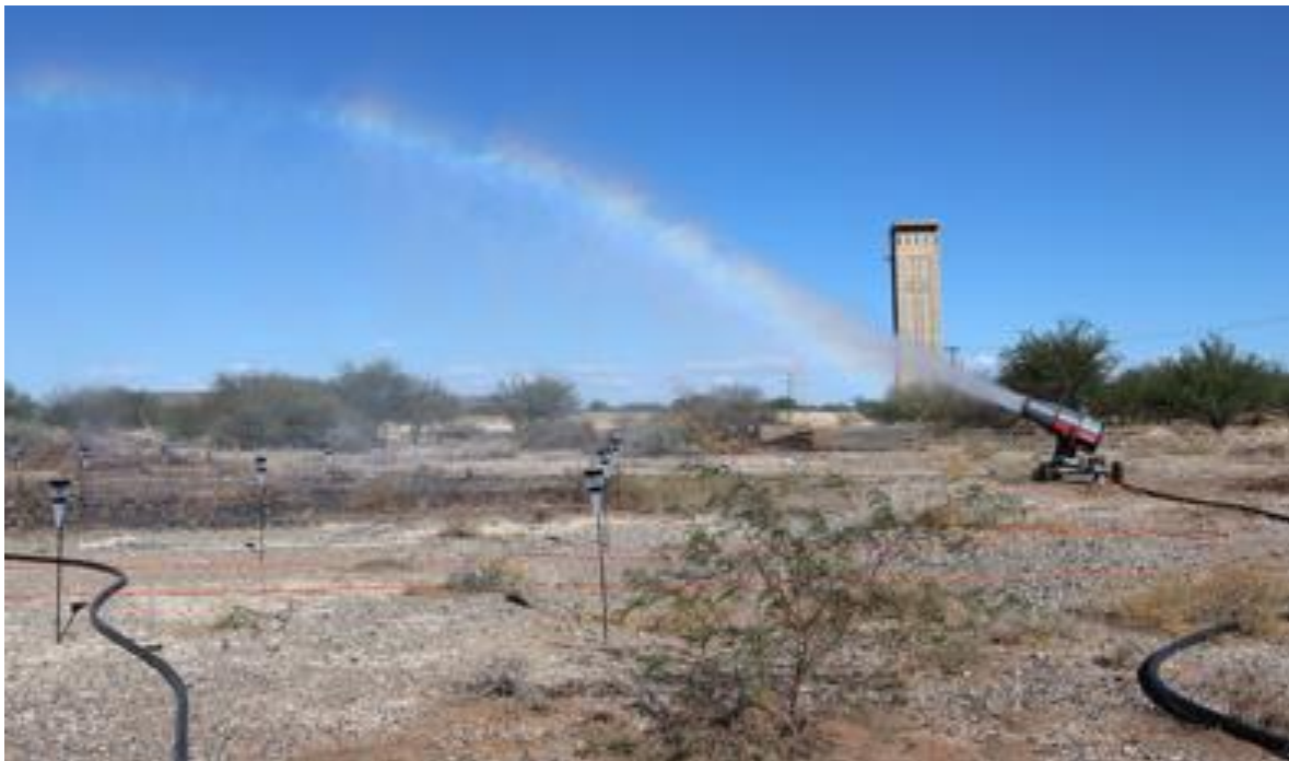
Figure 4: Feasibility study field trial of effectiveness of a 15kW evaporator at the Prieska Copper Zinc Project. The planned pilot trials aim to test 75kW and 90kW units as the next phase of the program.
