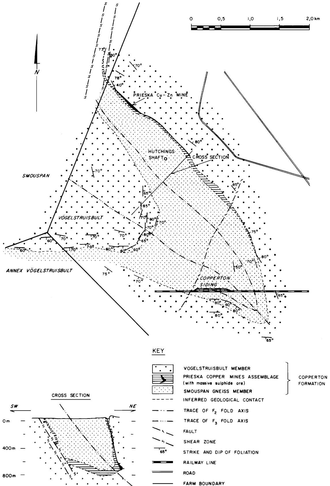
FIG. 6. Geologic map and section of the Prieska Zn-Cu deposit.
