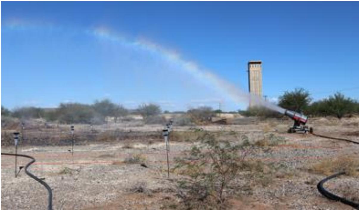
**Figure 5: Feasibility study field trial of effectiveness of a 15kW evaporator at the Prieska Project. The planned pilot trials aim to test 75kW and 90kW units as the next phase of the program.**
